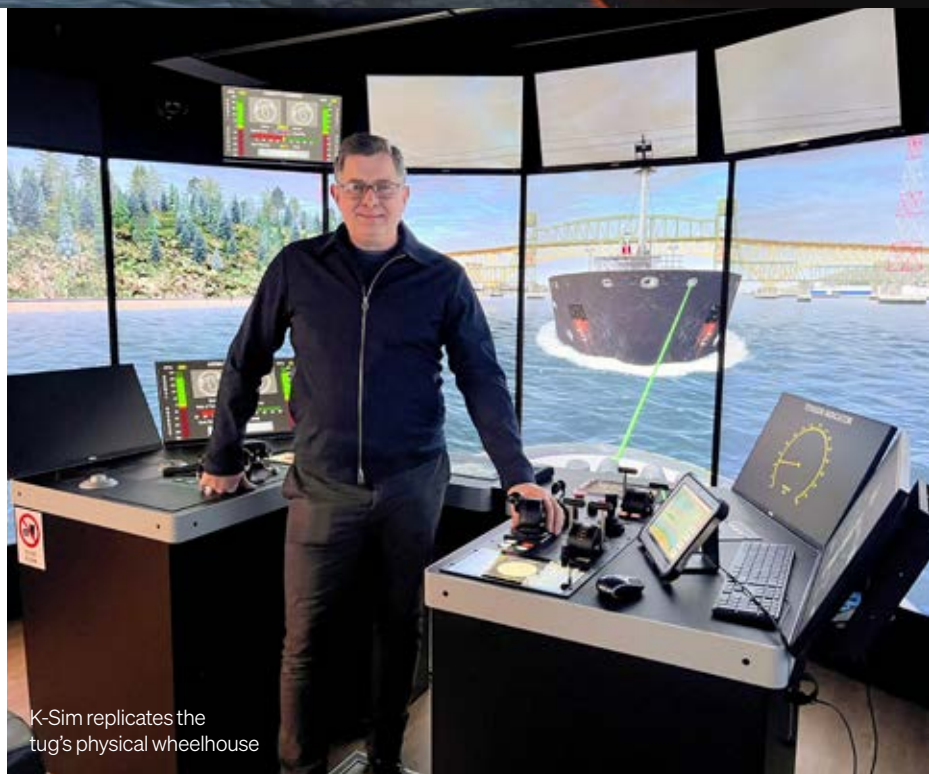
K-Sim allows operators to practice tug handling, such as escorting a large container vessel
